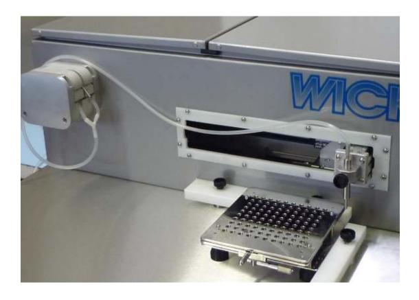
The filling assembly for hardshell gelatine capsules as well as for vegetarian capsules can be attached to the most of common manual powder capsule filling systems.
