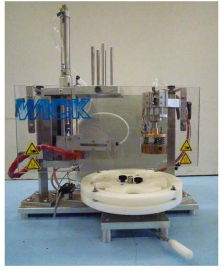
With manual rotary indexing table and automatic foil dispenser. Excellently suitable for sealing plastic jars and cups with aluminium foil.
