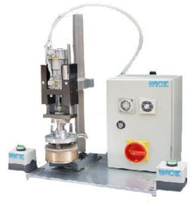
Excellently suitable for sealing plastic jars and cups with aluminium foil.
