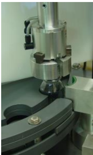
gripper style capping head for secure capping
