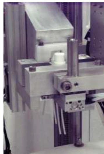
applicator for spray pumps incl. tensioning the tube
