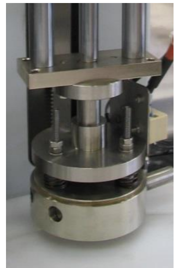
hot sealing station
